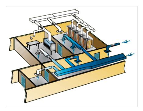
2. Because the racks are connected to the negatively pressurized exhaust system, this fresh air (blue arrows) is drawn into cages through their inlet filters at the appropriate flow rate to maintain the cage at the same temperature and relative humidity as the room.
