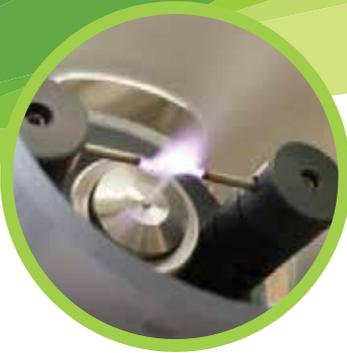
BIT Solution converts to **IHP** after passing through an atmospheric cold plasma arc breaking the double bond of the H<sub>2</sub>O<sub>2</sub> and creating Hydroxyl Radicals..
